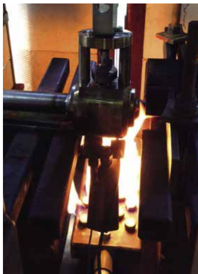
Valve during Fire Testing
